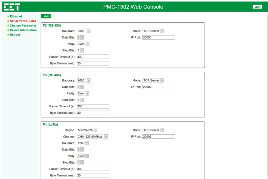
Figure 4-6 Serial Port & LoRa Settings
