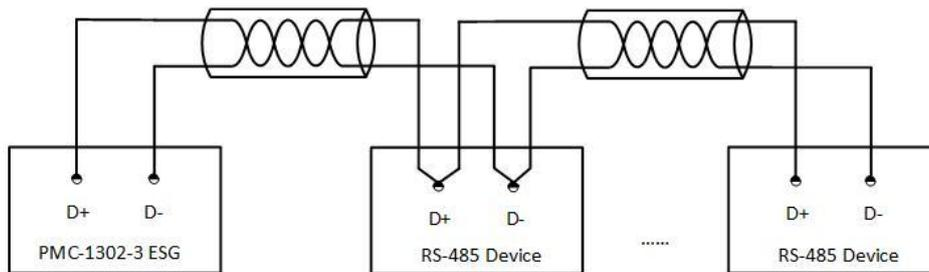
Figure 2-5 S485 Communications Connections
