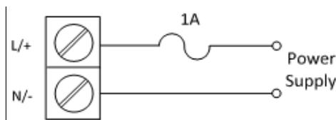
Figure 2-6 Power Supply Connections
